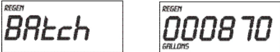
**Additional Features** - The Culligan Platinum Series Softener electronics are packed with features that expand the water softening experience. The statistics button allows you to view four separate gages: Capacity Remaining, Water Used Today, Average Water Usage, and Current Flow Rate. To view each item, press the statistics button, to step to the next item, press the button again. These screens will time-out after 5 seconds if no button is pushed.
