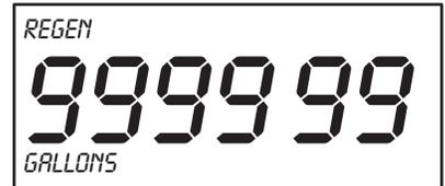
17. **Additional Features** - The Culligan Gold Series Softener electronics are packed with features that expand the water softening experience. The statistics button allows you to view four separate gages: **Capacity Remaining, Water Used Today, Average Water Usage, and Current Flow Rate.** To view each item, press the statistics button, to step to the next item, press the button again. These screens will time-out after 5 seconds if no button is pushed.
