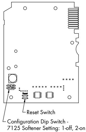
Rear View of Interface Circuit Board
