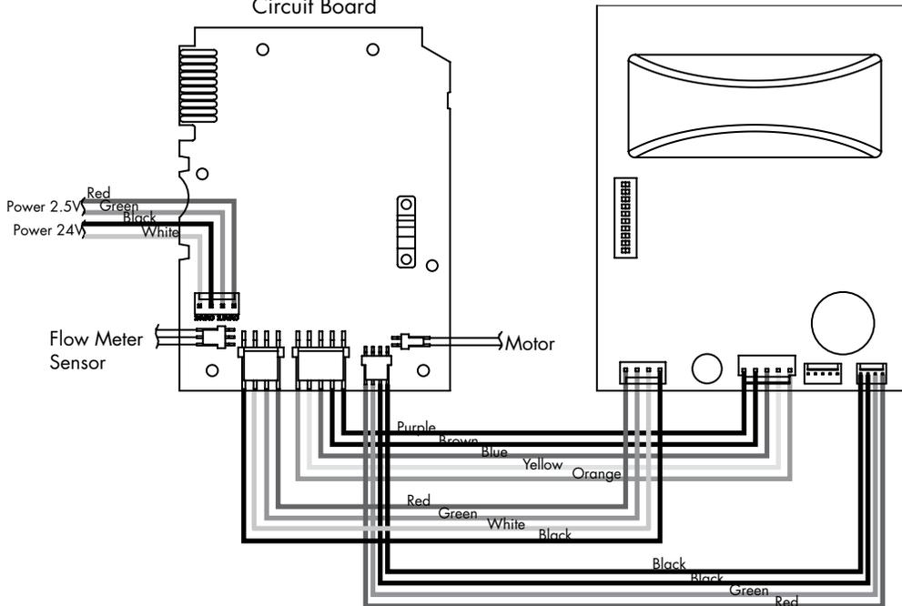
Motor and power wires are not polarity sensitive
